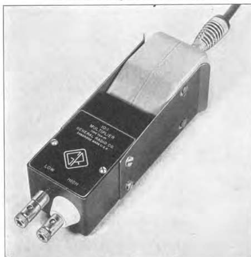
FIGURE 1. The voltmeter probe plugs into the 1500-volt multiplier as shown here.
